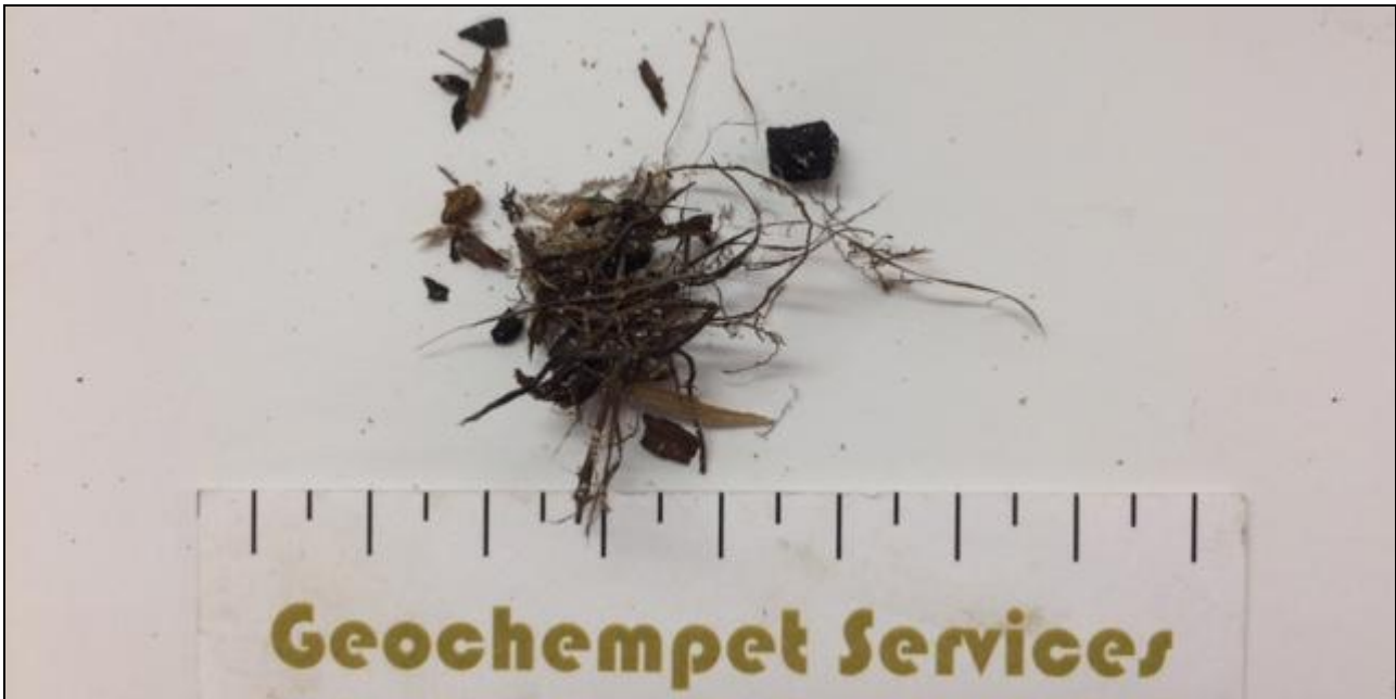
Figure 3: Image of the coarse fraction showing plant fragments and charcoal.
