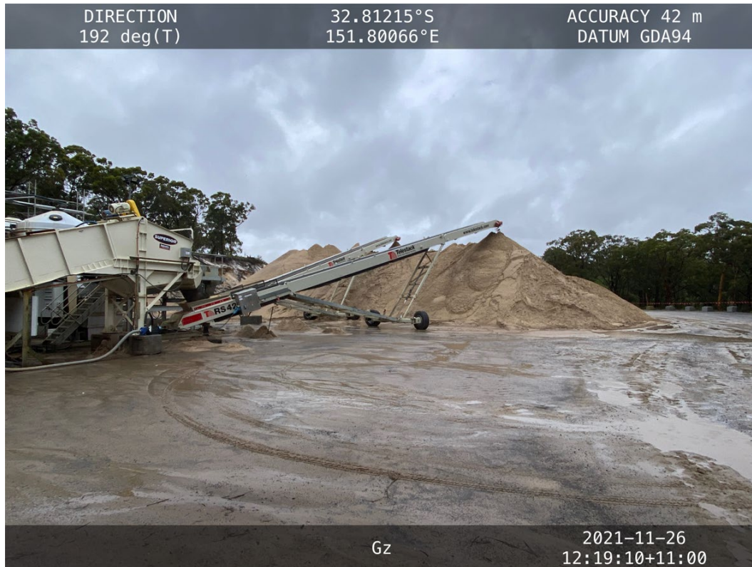
Photograph 8: Wash plant conveyors stacking washed sand for sale, note water in fore ground from rainfall.
