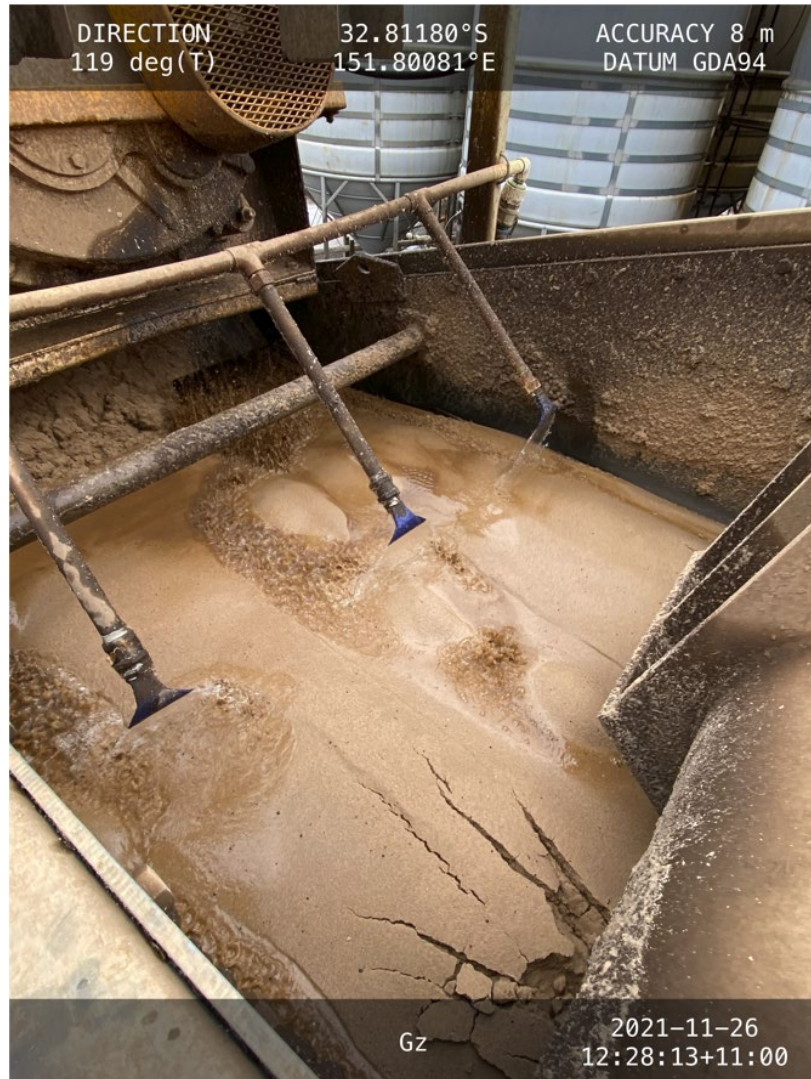
Photograph 7: Wash plant shaker table, reducing water take and product sand moisture content
