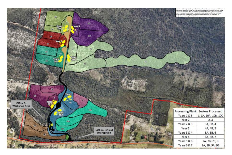
Figure 2 – Proposed site layout and sequence of sand extraction
